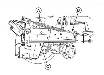
Figure 17. Lift Assist Spring
